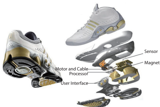
Adidas 1 Sole Breakdown Structure (source: www.aididas.com )
