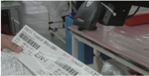
Picture 1 Through scanning the barcode of parts to collect information and reduce human errors in copying.
